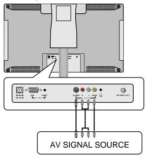
After connection, turn on the power of the unit and the external AV signal source and then press the INPUT button to shift to COMPOSITE or S-VIDEO mode.
